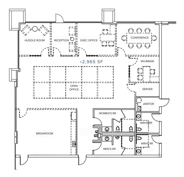
Note: Dashed lines (= = = =) indicate potential future office plan and will not be constructed in the shell building
